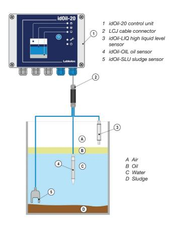
Connection with three sensors, two relays and supply voltage
