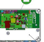
fault LED light up green. Push the button (7) on the top PCB briefly. The automatic sensor detection starts and the fault LED (4) flashes green. Attach the front cover and lock it in place with the four plastic screws. After all connected sensors have been detected, the corresponding
